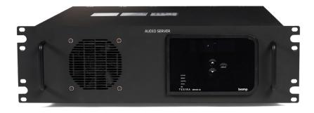
The Audio Server is a repackaged commercial off-theshelf (COTS) Digital Audio Network Server that provides automatic mixing, gain control, gating, and acoustic echo cancellation for VTC headsets and a CODEC. Multiple CODEC interface configurations are possible.
